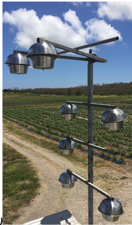
Figure 2-Pole Assembly for the Passive Air Samplers(PAS)
