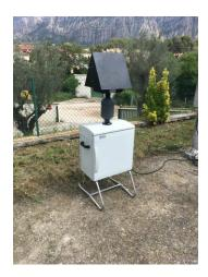
Sampling period might vary depending on the air sampler employed. In the particular case of high volume samplers, sampling collection could be accomplished in 24 h at a flow of de 45  $m^3/h$ . In case that the apparatus is not capable of acquiring this flow, smaller flows can be
