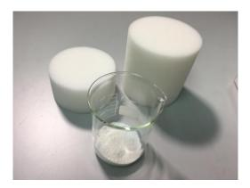
First step consists in placing the smaller PUF inside the glass holder, followed by 10 g of the polymer resin (XAD-2) and finally the larger PUF to cover and sealing the system.
